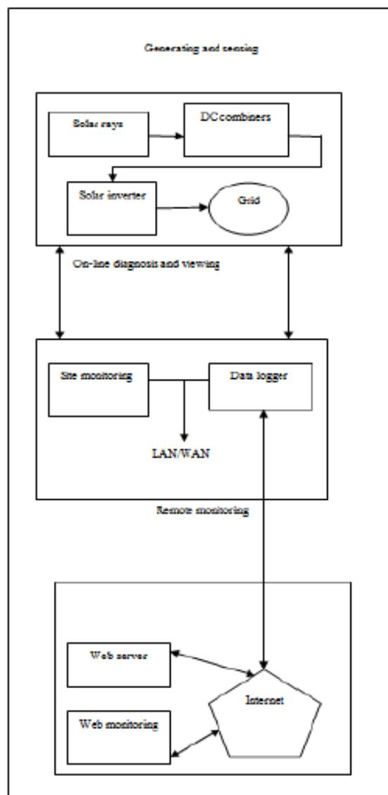
Fig. 3. Three-level monitoring of photovoltaic Power systems based on wireless communication
